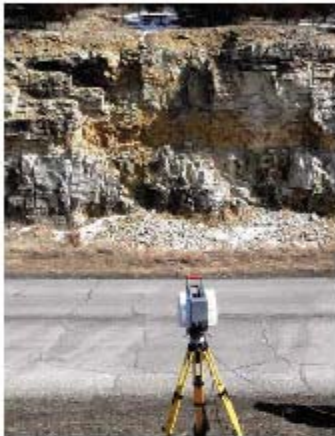
Figure 1: LIDAR scanner measuring rock cut
